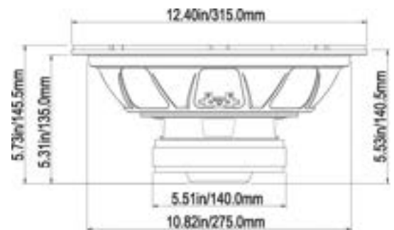
Recommended Air Space Sealed 1.15 cu. ft. / Vented 1.42 cu. ft.
